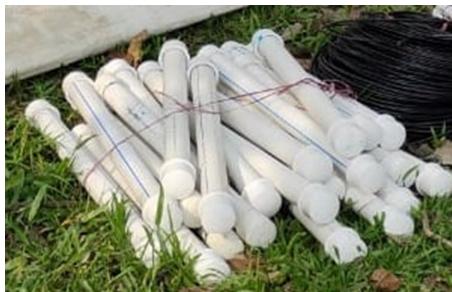
F: (i) 6 mm Gym cable & 2.54 cm diameter UPVC pipe (ii) Pierce holes at both ends and the centre
