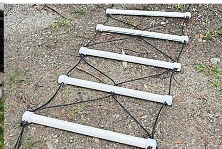
F: (i) 6 mm Gym cable & 2.54 cm diameter UPVC pipe (ii) Pierce holes at both ends and the centre
