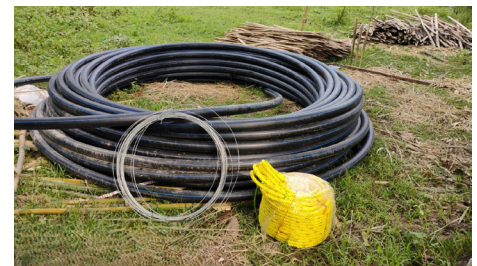
E: High-density polyethylene (HDPE) pipes (6.08 cm diameter, typically used for water supply), 2.4 cm diameter nylon rope and 4 mm galvanised wire.
